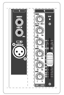
Fig. 2.1: Connectors and controls on the mono channels
