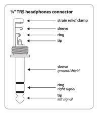
Fig. 4.4: Stereo plug for headphones connection
