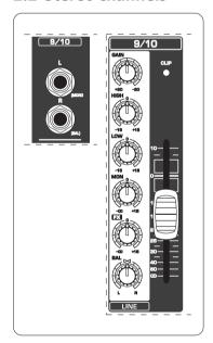
Fig. 2.2: Connectors and controls on the stereo channels
